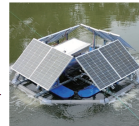
Solar Micro-pore Aerator Installation Site
