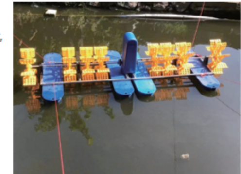
Waterwheel Aerator Installation Site
