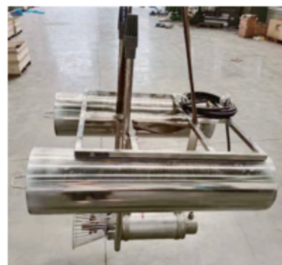
Solar Push-flow Aerator
