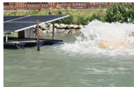
Solar Spring Aerator Installation Site
